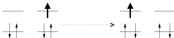
Figure 3. The nearest-neighbour hopping process for the P-LC assisted by the F-LC.
